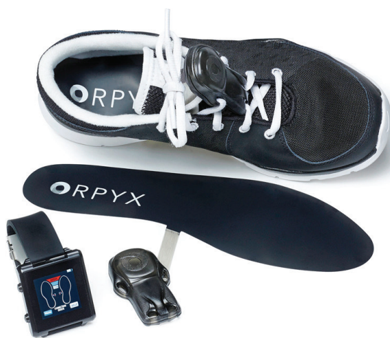
The SurroSense Rx system (shoes not included). Image courtesy of Orpyx Medical Technologies. 15
