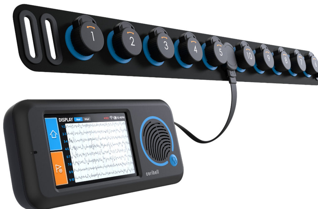
Figure 1: Ceribell EEG Headband and Recorder
